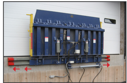
Roller trolley assembly allows for lateral movement to accommodate the position of the rail car.
