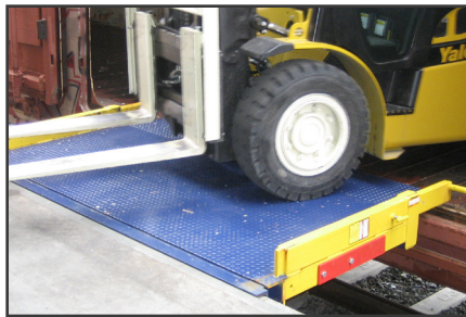
Standard yellow run-off guards to help prevent a forklift truck from driving off the edge.
